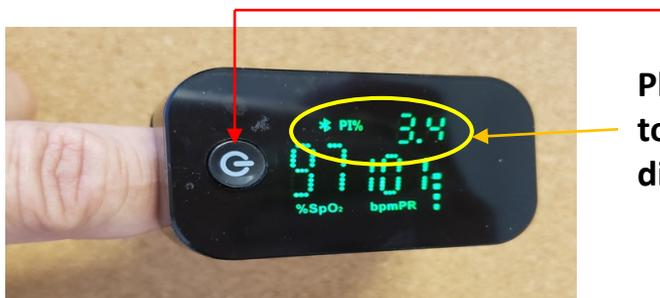
Place the finger properly and turn on the **power button** to begin, measurement is complete once the **PI** is displayed.
