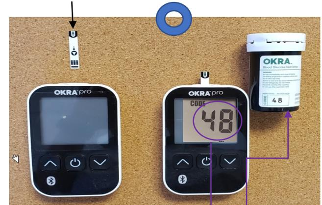
Power turns on when the test strip is inserted then displays the matching strip code on the screen. Once the code disappears, blood can be drawn.
